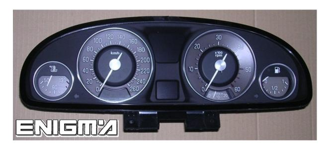
USE CABLE C4, REMOVE DASH FROM CAR, OPEN BACK COVER, PLEASE MAKE IT CAREFULLY. REMOVE UPPER BOARD. WHEN WE CAN SEE THE MAIN BOARD LOCATE EEPROM MEMORY, AND CLIP IT AS SHOWN OF PHOTO BELOW:
