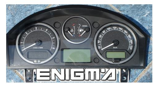
USE CABLE C4, OPEN BACK COVER FROM DASH, LOCATE EEPROM M35080 MEMORY AND CLIP IT CHECKING PIN 1 AS SHOWN OF PHOTO BELOW:
