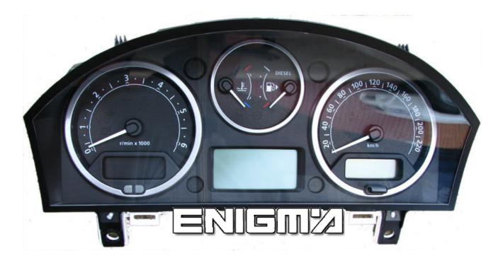
USE CABLE C4, OPEN DASH AND LOCATE EEPROM 35080 MEMORY. NOW ONLY CLIP IT CHECKING PIN 1 AS SHOWN ON PHOTO BELOW:
