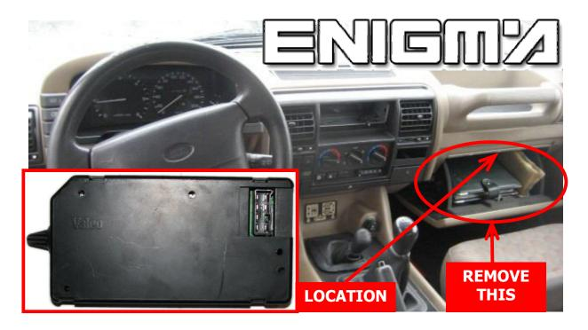
USE CABLE C11, REMOVE THIS UNIT, IT IS NOT DIFFICULT BUT TAKE YOUR TIME. OPEN IT ALL, PLEASE MAKE IT CAREFULLY, THEN CONNECT OR SOLDER CABLE LEADS ACCORDING TO COLOURS AS SHOWN OF BELOW PHOTOS:
