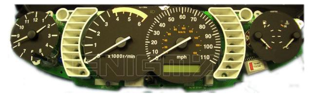
USE CABLE C11, REMOVE BACK COVER FROM DASH, THEN CONNECT OR SOLDER CABLE LEADS ACCORDING TO COLOURS AS SHOWN ON PHOTO, REMEMBER TO LIFT UP ONE PIN FROM MICRO:
