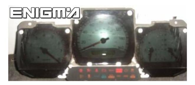
USE CABLE C4, OPEN BACK SIDE FROM DASH, CAREFULLY, THEN LOCATE EPROM 93C46, AND CLIP IT CHECKING PIN 1 AS SHOWN OF BELOW PHOTO:
