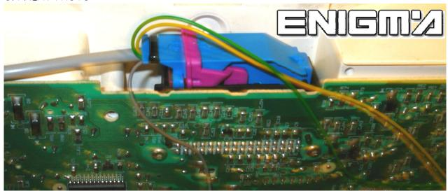
AND THEN CONNECT OR SOLDER CABLE LEADS ACCORDING TO COLOURS AS SHOWN ON THE PHOTO BELOW:
