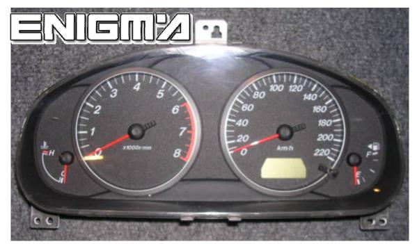
Use cable C4, open all dash, but we must take carefully, we must remove nails, then locate eprom 93C56, and clip it checking Pin 1 as shown of below photo:
