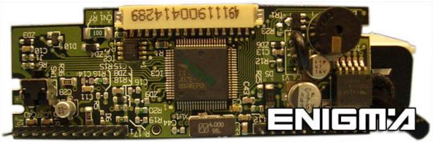
NOW LOCATE EPROM 93C46, AND CLIP IT CHECKING PIN 1 AS SHOWN ON PHOTO BELOW:
