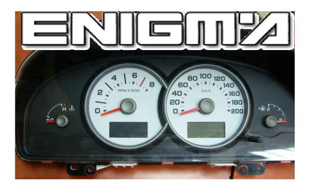
USE CABLE C12, OPEN BACK COVER FROM DASH, CAREFULLY, THEN CONNECT OR SOLDER CABLE LEADS ACCORDING TO COLOURS AS SHOWN OF BELOW PHOTO:
