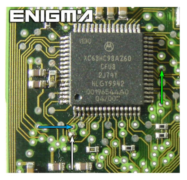
IF MICRO MASK IS 1J35D OR 3J74Y OR 4J74Y, WE MUST USE PHOTO BELOW, REMEMBER TO SOLDER RESISTOR OF 10K TO GREY CABLE:
