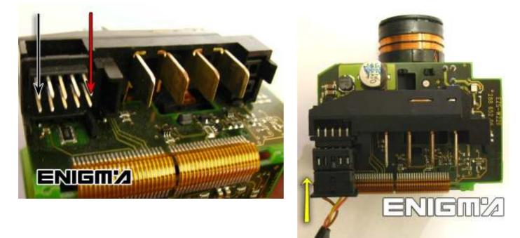
THEN SOLDER CABLE LEADS ACCORDING TO COLOURS AS SHOWN ON THE PHOTO BELOW:
