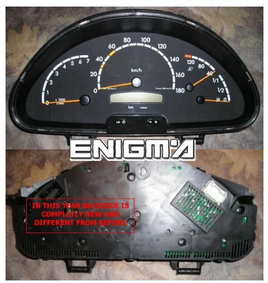
USE CABLE C4, OPEN BACK PART OF DASH, BE CAREFULL, THEN LOCATE EPROM 93C66, AND CLIP IT CHECKING PIN 1 AS SHOWN OF BELOW PHOTO:
