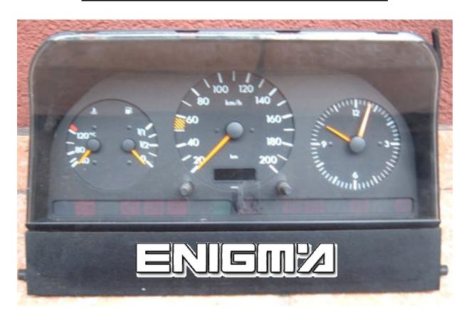
USE SPECIFIC CABLE C32, REMOVE DASH FROM CAR, AND CONNECT PLUG TO DASH LIKE WE CAN SEE ON NEXT PHOTO AND RUN PROGRAM:
