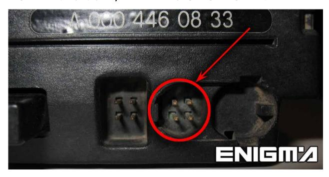
USE SPECIFIC CABLE C33, CONNECT PLUG TO DASH LIKE WE CAN SEE ON PHOTO BELOW AND RUN PROGRAM:
