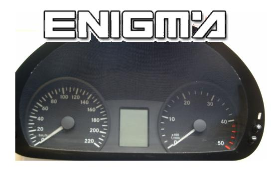
USE CABLE C4, OPEN ALL DASH, PLEASE MAKE IT CAREFULLY, SPEACILLY CAREFUL WITH SCREEN. THEN LOCATE EPROM MEMORY 25C640, WE DON'T NEED TO DESOLDER IT, AND CLIP IT CHECKING PIN 1 AS SHOWN OF PHOTO BELOW:
