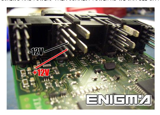
THEN SOLDER CABLE LEADS ACCORDING TO COLOURS AS SHOWN ON THE PHOTO BELOW:
