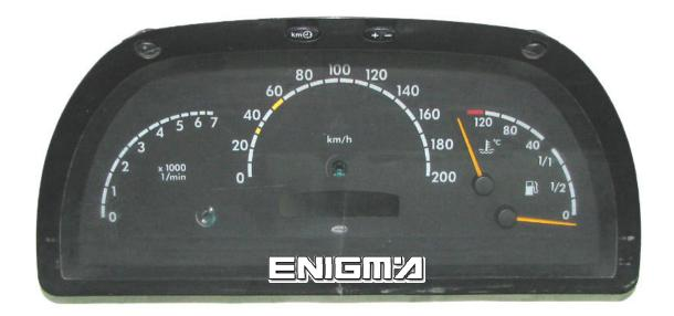
USE SPECIFIC CABLE C31, REMOVE DASH FROM CAR, CONNECT PLUG TO DASH LIKE WE CAN SEE ON NEXT PHOTO AND RUN PROGRAM:
