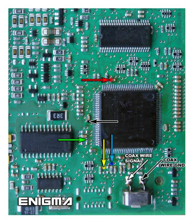
3. TO WORK ON CAS3+, WE MUST USE CABLE C45 + A6 ADAPTER. REMOVE MODULE FROM CAR CAREFULLY, OPEN IT, AND LOCATE POINTS ON THE BOARD AND SOLDER CABLE LEADS:
