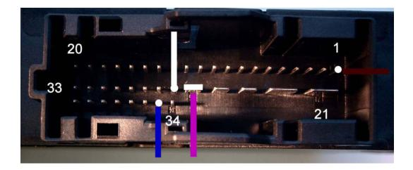
CAS PIN 25 - ENIGMA DB25 PIN 03 GND CAS PIN 35 - ENIGMA DB25 PIN 08 CAN CAS PIN 26 - ENIGMA DB25 PIN 21 CAN CAS PIN 01 - ENIGMA DB25 PIN 25 +12V 2. TO WORK ON CAS3, WE MUST USE CABLE C45 + A6 ADAPTER. REMOVE MODULE FROM CAR CAREFULLY, OPEN IT, AND LOCATE POINTS ON THE BOARD AND SOLDER CABLE LEADS:
