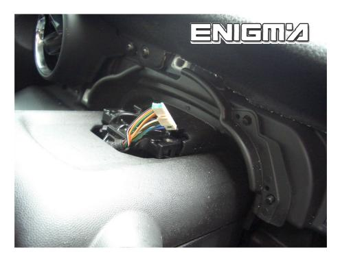
If you follow the wire that goes into the dash you will see BMW style connector. Using cable C40, plug your tool into here as shown of photo below:
