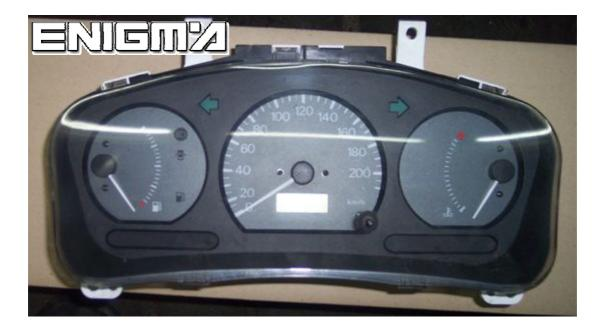
Use C5 cable, take off only speedometer, it is the screen one, then we can see the 93C46 eprom, and with the photo below we can clip memory or we can choose to make by back soldering cable for it C7:
