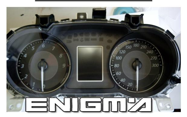
USE C7 CABLE, WE ONLY NEED TO REMOVE BACK PLASTIC COVER FROM DASH, LOCATE POINTS IN THE MAIN BOARD LIKE IN PHOTO BELOW AND SOLDER CABLE LEADS AS IT SHOWS TO US. NEVER TOUCH NAILS. MEMORY INSIDE THOSE KINDS OF CARS IS A 93C86.
