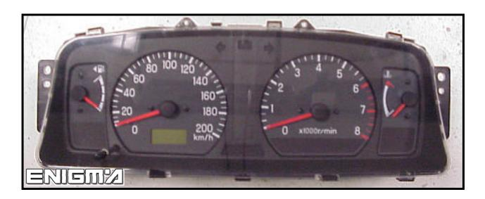
USE C7 CABLE, TAKE OFF ONLY SPEEDOMETER, IT IS THE SCREEN ONE, THEN WE CAN SEE THE 93C46 EPROM, AND WITH THE PHOTO BELOW WE CAN CLIP MEMORY OR WE CAN CHOOSE TO MAKE BY BACK SOLDERING CABLE FOR IT C7:
