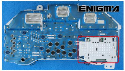
OPEN AND LOCATE EPROM 93C56, SOMETIMES MUST BE CLENED, AND CLIP IT CHECKING PIN 1 AS SHOWN IN THE PHOTO BELOW:
