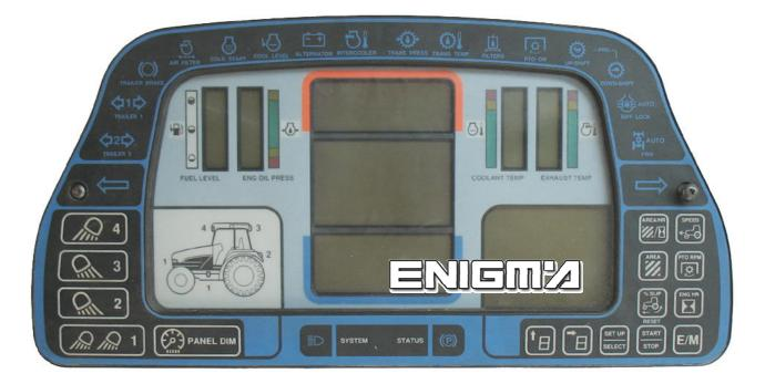
Use cable C4, open dash, please make it carefully, then locate eeprom 93C66 memory and clip it checking pin 1 as shown of photo below:
