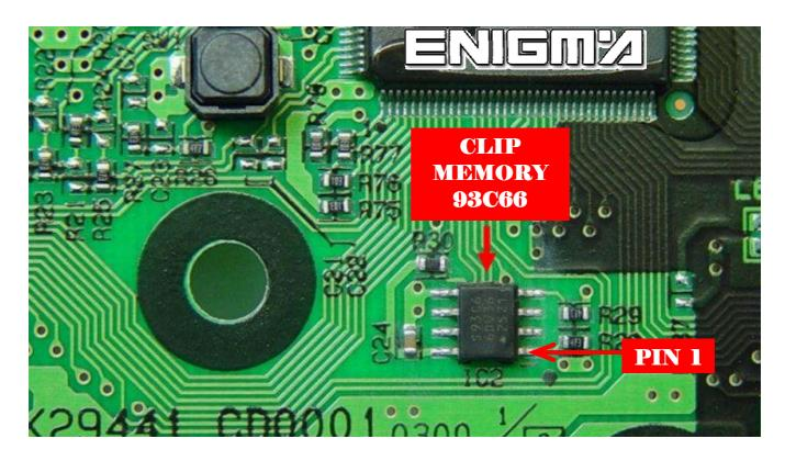
ALTHOUGH WE CAN USE METHOD LIKE IN ALL NISSAN SOLDERING POINTS BY BACK, HERE YOU HAVE RIGHT CONNECTION FOR LEADS USING CABLE C7:
