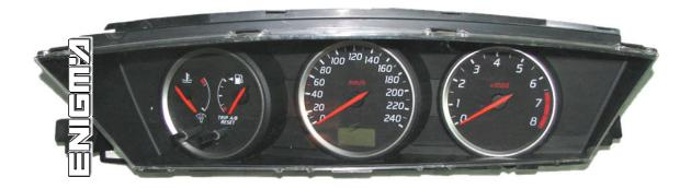
USE CABLE C4, OPEN DASH, PLEASE MAKE IT CAREFULLY, THEN LOCATE EEPROM 93C66 MEMORY AND CLIP IT CHECKING PIN 1 AS SHOWN OF PHOTO BELOW:
