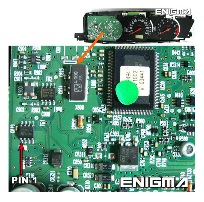
WE CAN ALSO USE C7 CABLE, WE ONLY NEED TO REMOVE BACK PLASTIC COVER FROM DASH, LOCATE POINTS ON THE MAIN BOARD, LIKE IN PHOTO BELOW, AND SOLDER CABLE LEADS AS IT SHOWS TO US:
