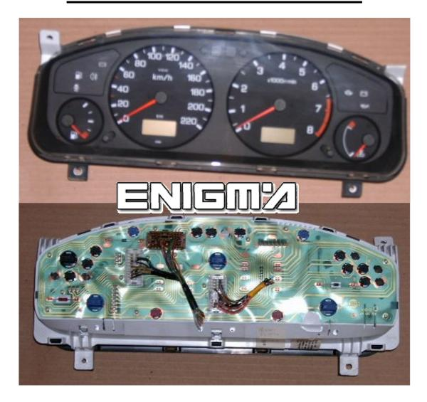
USE CABLE C4, REMOVE FRONT PLASTIC COVER, TAKE OFF SPEEDOMETER, ONLY FIXING WITH 4 SCREWS. THEN LOCATE EPROM MEMORY 93C46, THAT WE MUST DESOLDER, CLIP IT CHECKING PIN 1 AND RESOLDER AS SHOWN OF PHOTO BELOW:
