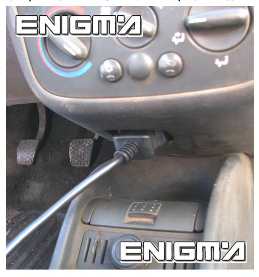
SELECT FROM MENU PROGRAM OPEL CORSA C DIAG. NOW READ ACTUAL KM, AFTER SELECT NEW KM AND ENTER NEW VALUE. DURING PROGRAMATION BUTTON FROM DASH MUST BE HOLDED. CHECK PHOTO BELOW:
