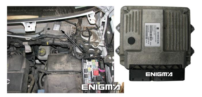
USE CABLE C4, REMOVE ECU FROM CAR, OPEN IT CAREFULLY, ON THE BOARD'S HIDDEN SIDE WE CAN LOCATE EPROM, CLIP IT AS YOU CAN SEE ON BELOW PHOTO:
