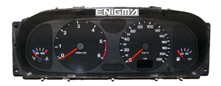
USE CABLE C4, HIGH CAREFULLY TO REMOVE NAILS FROM THIS DASH WHEN YOU WANT TO CLIP THE EPROM MEMORY. IT IS A VERY STRANGE MEMORY WITH A DIFFERENT CODE AS USUAL, MADE BY ATMEL, BUT EQUAL AS A SIMPLE 93C46, WHEN WE HAVE MAIN BOARD CLIP IT CHECKING PIN 1 AS SHOWN OF PHOTO BELOW:
