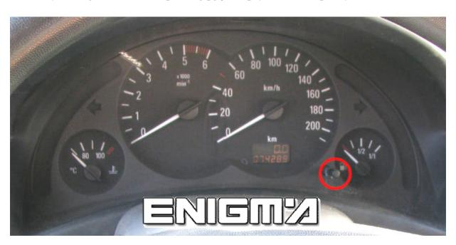
AFTER REPROGRAMATION DISCONNET THREE FUSES (YOU CAN SEE WHICH ONES ON NEXT PICTURE) FOR AROUND 15 SECONDS AND CONNECT IT BACK.
