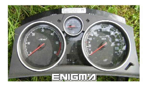
USE CABLE C4, OPEN ALL DASH, BUT WE MUST TAKE MUCH CAREFULL, WE MUST TAKE OFF NAILS, AND LEAVE SCREEN FIX TO THE MAIN BOARD, THEN LOCATE EPROM M35080, AND CLIP IT CHECKING PIN 1, WE CAN SEE LOCATION ON PHOTO BELOW:
