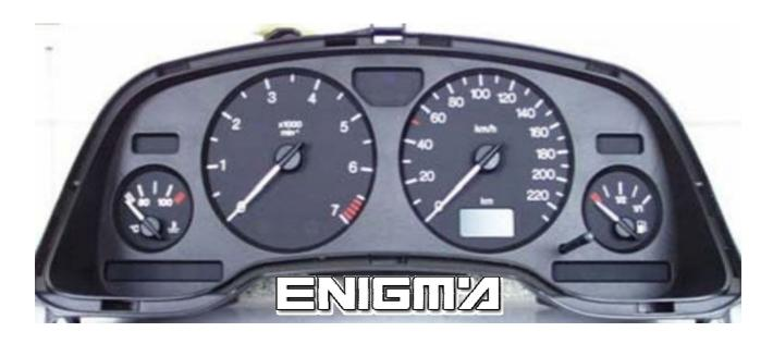
USE CABLE C4, OPEN ALL DASH, BUT WE MUST TAKE MUCH CAREFULL, WE MUST TAKE OFF NAILS, THEN LOCATE EPROM 24CO2 MEMORY, AND CLIP IT CHECKING PIN 1 AS SHOWN ON PHOTOS BELOW:
