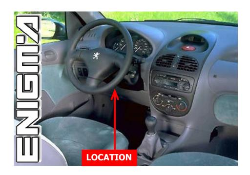
USE CABLE C4, REMOVE BACK PLASTIC COVER FROM BSI, THEN LOCATE EEPROM AND CLIP IT CHECKING PIN 1 AS SHOWN OF PHOTO BELOW:
