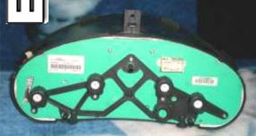
USE CABLE C4, OPEN ALL DASH, PLEASE MAKE IT CAREFULLY, ENGINES ARE VERY FRAGILE WHEN YOU TRY TO REMOVE NAILS. THEN LOCATE EPROM MEMORY 95020, USUALLY WE DON'T NEED TO DESOLDER IT.
