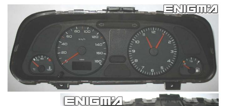
USE SPECIFIC CABLE C24, REMOVE DASH FROM CAR, CONECT PLUG TO DASH LIKE WE CAN SEE ON PHOTO AND RUN PROGRAM:
