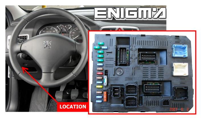
USE CABLE C4, REMOVE BACK PLASTIC COVER FROM BSI, THEN LOCATE EEPROM AND CLIP IT CHECKING PIN 1 AS SHOWN OF PHOTO BELOW:
