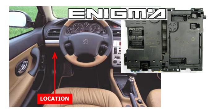
Use cable C4, take off back side from BSI, and locate Eeprom memory 93C66 and clip it checking Pin 1 as shown of photo below:
