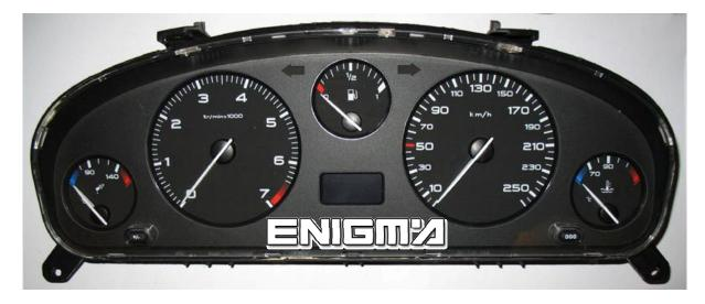
USE CABLE C4, OPEN DASH, PLEASE MAKE IT CAREFULLY, THEN LOCATE EEPROM 93C66 MEMORY AND CLIP IT CHECKING PIN 1 AS SHOWN OF PHOTO BELOW:
