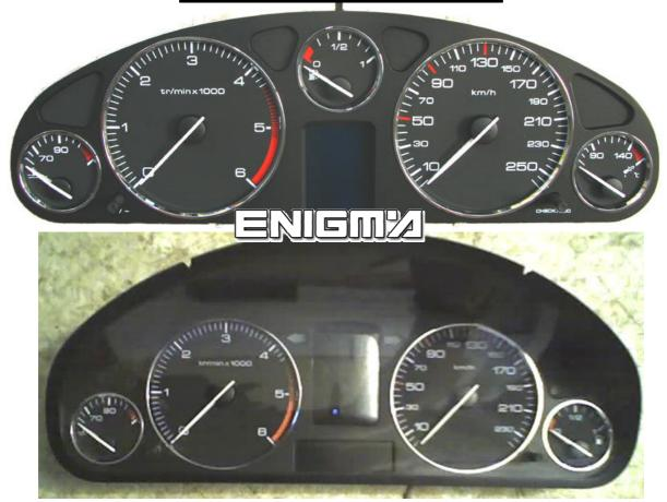
USE CABLE C4, OPEN DASH, PLEASE MAKE IT CAREFULLY, THEN LOCATE EEPROM 93C66 MEMORY AND CLIP IT CHECKING PIN 1 AS SHOWN OF PHOTO BELOW:
