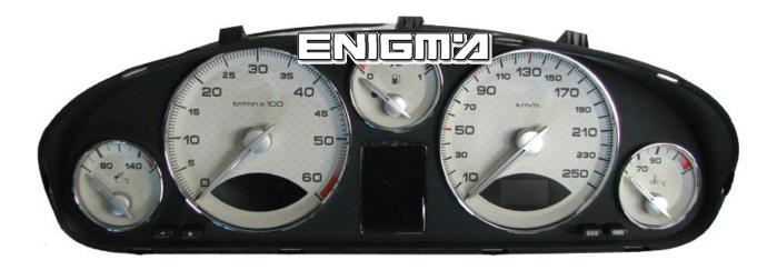
Use cable C4, open dash, please make it carefully, then locate eeprom 93C66 memory and clip it checking PIN 1 as shown of photo below:
