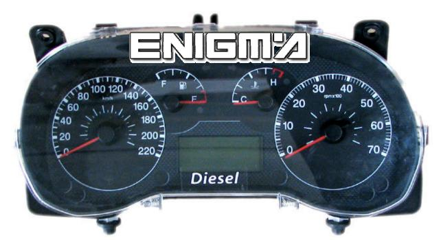
USE CABLE C4, REMOVE DASH FROM CAR, OPEN ALL DASH, PLEASE MAKE IT CAREFULLY. WHEN WE HAVE MAIN BOARD ON OUR HANDS LOCATE EEPROM MEMORY, AND CLIP IT CHECKING PIN 1 AS SHOWN OF PHOTO BELOW:
