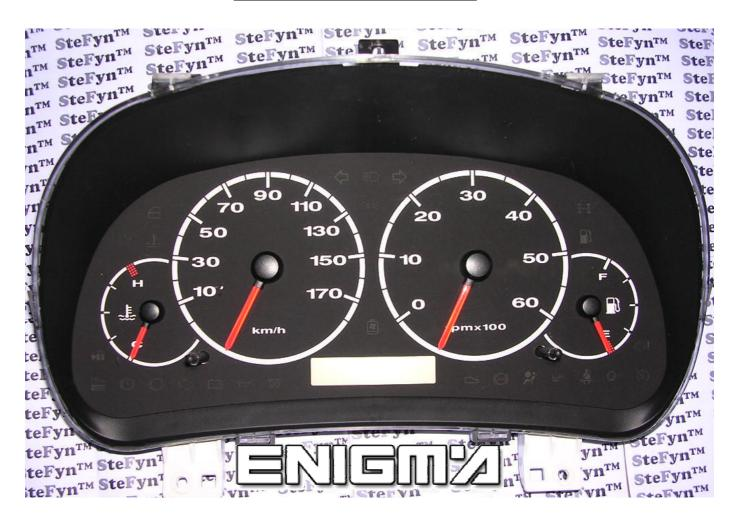
USE CABLE C4, OPEN ALL DASH, PLEASE MAKE IT CAREFULLY, LOCATE EPROM MEMORY 95040, USUALLY WE DON'T NEED TO DESOLDER IT, AND CLIP IT CHECKING PIN 1 AS SHOWN OF PHOTO BELOW:
