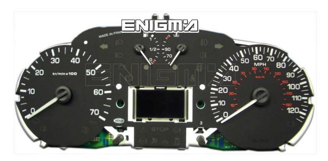
USE CABLE C4, OPEN DASH COMPLETLY, PLEASE MAKE IT CAREFULLY, NAILS HAVE A LITTLE DIFICULTY, BUT... WHEN WE HAVE ALL BOARD FREE IN OUR HANDS, LOCATE EEPROM 95020, SOMETIMES MUST BE DESOLDER, AND CLIP IT CHECKING PIN 1 AS SHOWN OF PHOTO BELOW:
