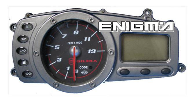
USE CABLE C4, OPEN OUTSIDE COVERS FROM DASH, THEN CUT A LITTLE WHITE INSIDE COVER AND WE CAN SEE THE EPROM MEMORY. NOW CLIP IT CHECKING PIN 1 AS SHOWN OF BELOW PHOTO:
