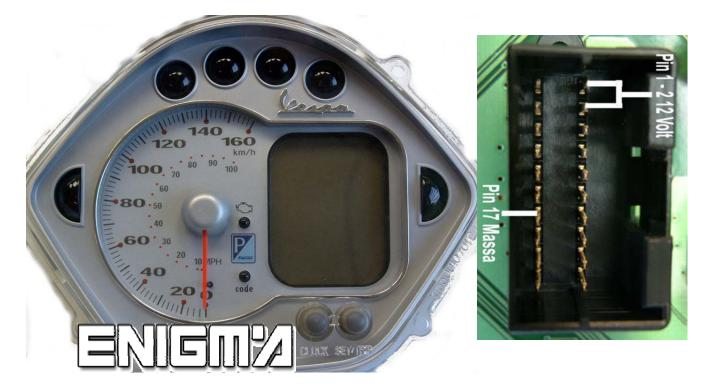
USE CABLE C4, REMOVE BACK PLASTIC COVER FROM DASH, THEN LOCATE EPROM 24C04, AND CLIP IT CHECKING PIN 1 AS SHOWN OF BELOW PHOTO:
