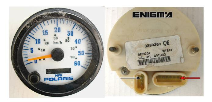
Use cable C4, take off dash from Quad, open all dash, please make it carefully. We must remove 3 screws under sticker. When we have main board on our hands locate eprom 93C46 memory, and clip it checking pin 1 as shown of photo below:
