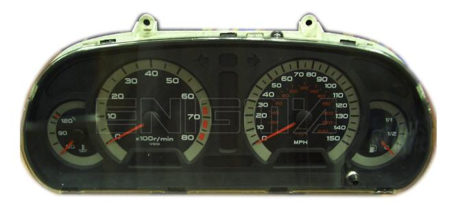
USE CABLE C4, OPEN DASH COMPLETELY, PLEASE MAKE IT CAREFULLY, AND LOCATE EEPROM 93S46 MEMORY. NEXT CLIP IT CHECKING PIN 1:
