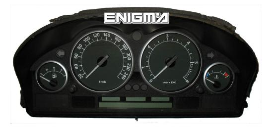
USE C7 CABLE, WE ONLY NEED TO REMOVE BACK COVER FROM DASH, IT IS DIFFICULT, MAKE IT CAREFULLY. LOCATE POINTS ON THE MAIN BOARD LIKE IN PHOTO BELOW AND SOLDER CABLE LEADS AS IT SHOWS TO US. NEVER TOUCH NAILS, IT IS VERY DANGEROUS. MEMORY INSIDE THOSE KINDS OF CARS ARE A M35080.
